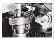
Valona 7035 IN is a chlorine free light coloured medium viscosity cutting oil compounded with active sulphur and fat to provide longer tool life and consistent surface finish.
